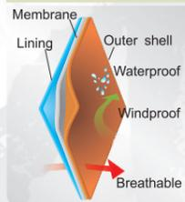
Membrane is bonded together with outer shell and lining.
