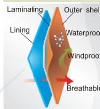
Fabric is treated with multi- micropores laminating.
