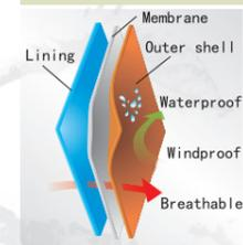
This symbol indicates Arctech membrane is applied as a separate layer between the shell and lining which facilitates noise reduction. Functional properties include wind stopper, waterproof and breathability. High quality protection for the hunting and outdoor enthusiast.
