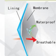
This symbol indicates membrane is two layers laminated with mesh backing. Breathable and low noise.
